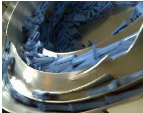
Feed rate = 200 pieces/min Part Name : Roller Clamp Orientation position : 1 Drive unit : RNA 630-1
