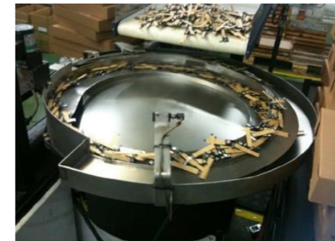
Cell Feeder running at 30 pcs/min. Bowl Diameter 800 mm
