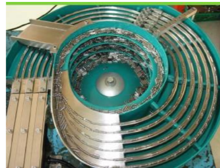
Feed rate = 20 pieces/min/track Part Name : Stop Pin No of tracks : 6 Drive unit : Customized
